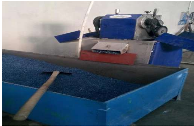
Figure 3. Granule production from plastic packaging waste
